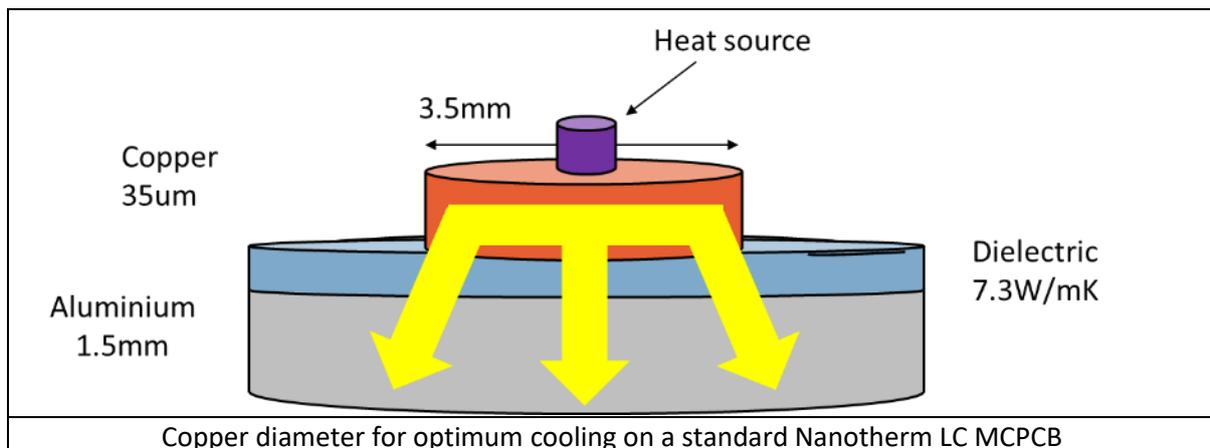
A common requirement is for the MCPCB to provide cooling to an array of components. In this instance there is a conflict between the layout for electrical function and the copper area required to remove heat effectively. A simple thermal design methodology is to proceed as follows:
