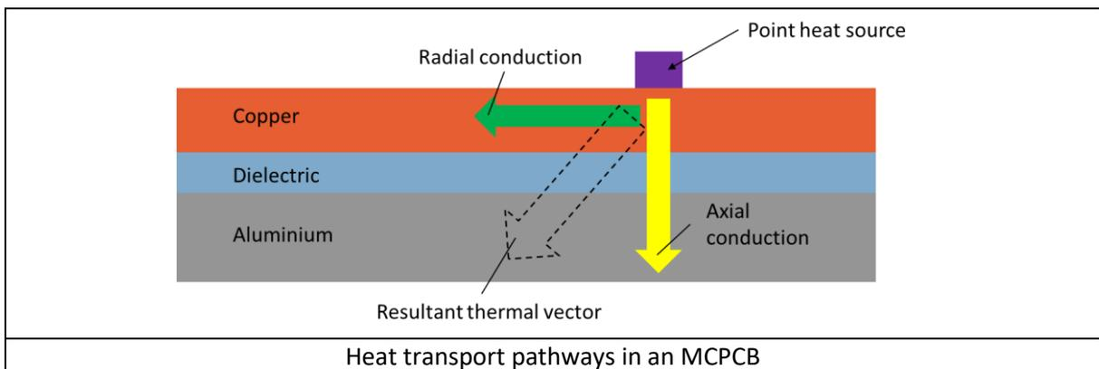
As can be seen from the above diagram, a large area of thick copper will be beneficial in extracting heat. But there are good technical and commercial reasons why thick copper should be avoided. In particular, thick copper:
