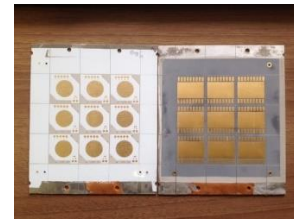
Processed tile, carrying one customer units, each of which contains nine circuits.
